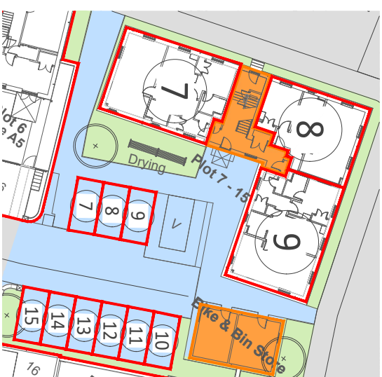
BLOCK 1 GROUND FLOOR PLAN
